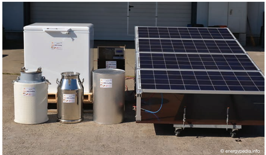
Photo 1. Example of a simple solution for milk can cooling. Solar panelled powered freezer, to rapidly cool down milk. © energypedia.info
